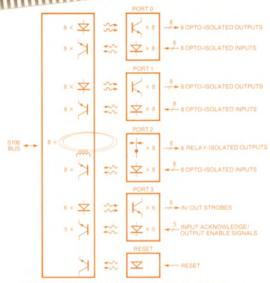
CROMEMOO 4PIO INTERFACE, NOTE THAT ALL I/O LINES ARE EITHER OPTICALLY OR MAGNETICALLY ISOLATED FROM THE COMPUTER CIRCUITS
