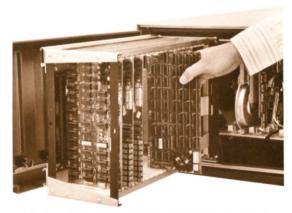
System Three computer is constructed so that hinged front panel swings open and mother-board/card cage slide out for easy insertion of circuit boards.
